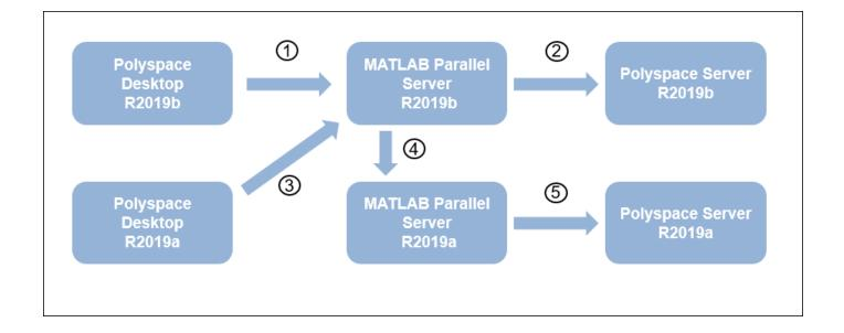
To support submissions from multiple releases with a single MATLAB Parallel Server cluster, you have to link the various installations of Polyspace products and MATLAB Parallel Server. Of the links shown in the preceding figure, the links numbered 1, 2 and 5 are part of a regular server-client installation using all products from the same release. To create all the links, do these steps:
